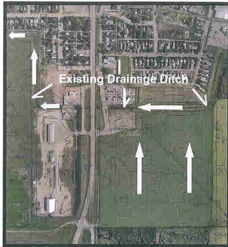
Figure 2 – Site Drainage – Southern Portion of Plan
